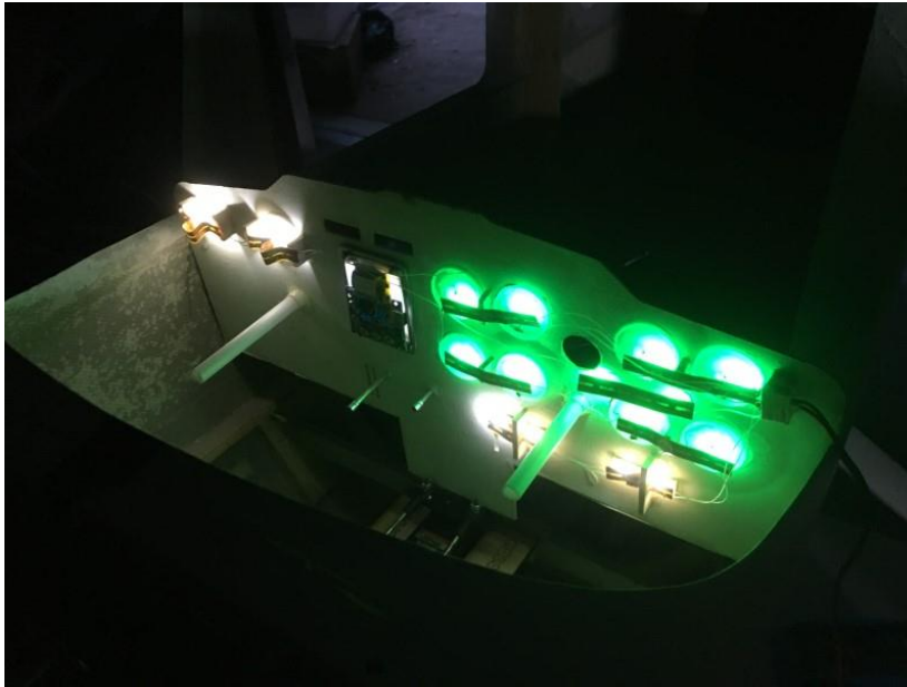
Back side of instrument panel showing the LED back lighting.
