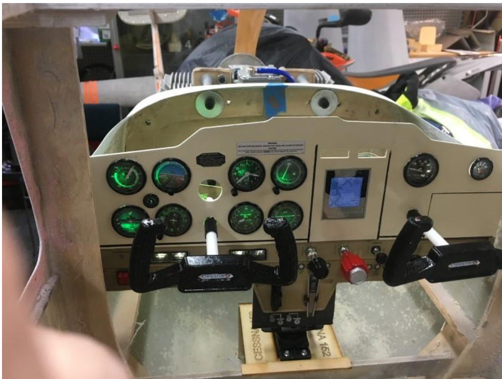
Back lighting of the instrument panel from the front Pilots view.
