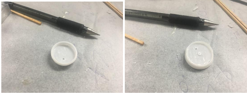
Front and rear view of the 3D printed instrument body with support structure removed
