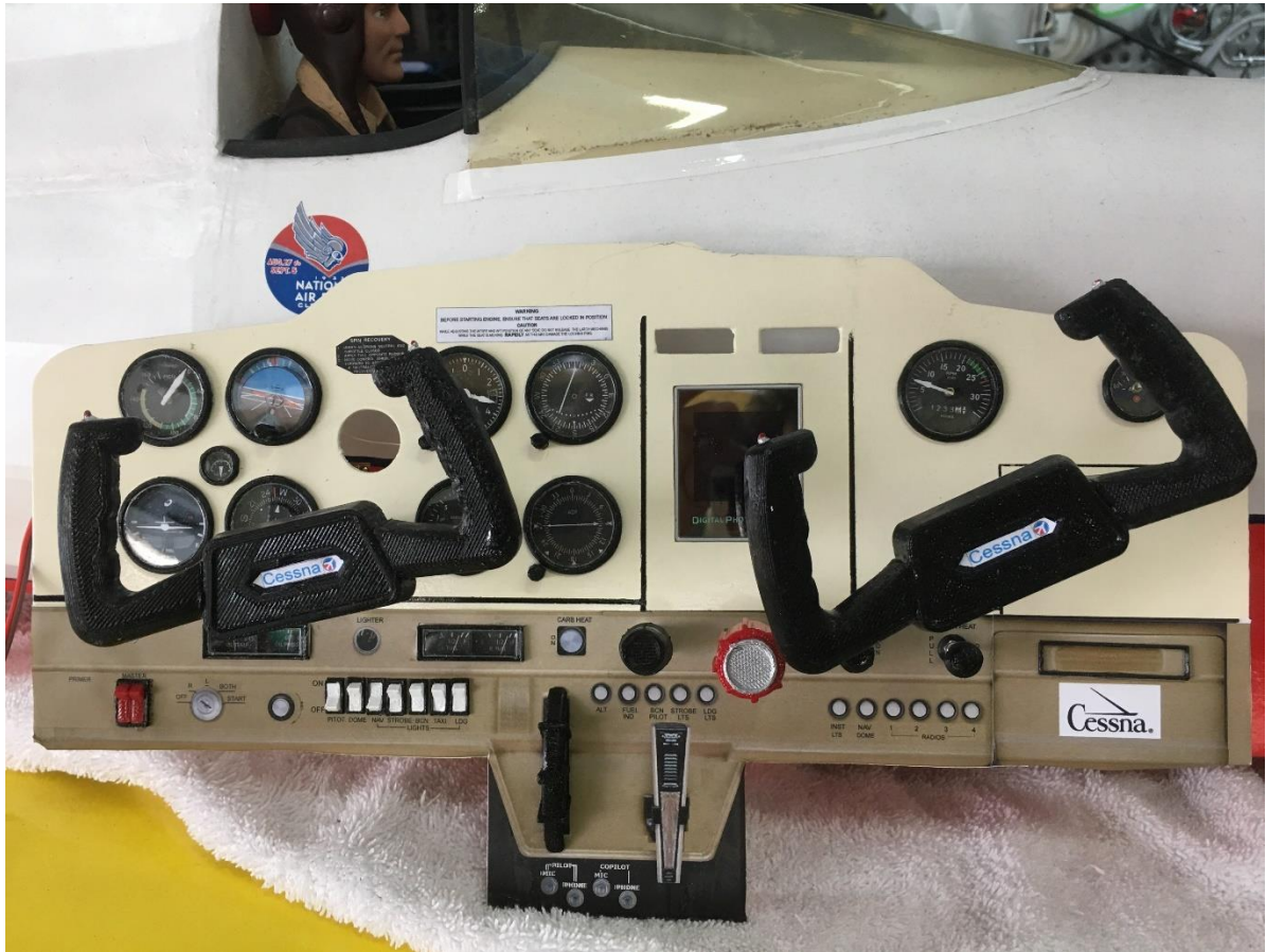
Nearly completed Cessna 152 instrument panel with additional 3D designed and printed parts such as switches and knobs.
