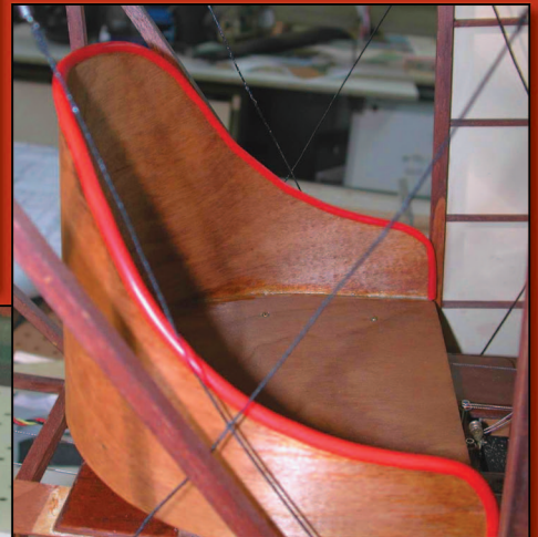
Top: Pilot's seat constructed from 0.3mm ply and stained and then glued together.
