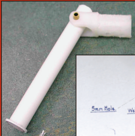
Aileron torque tube and control stick pivot manufactured using the 3D printer.
