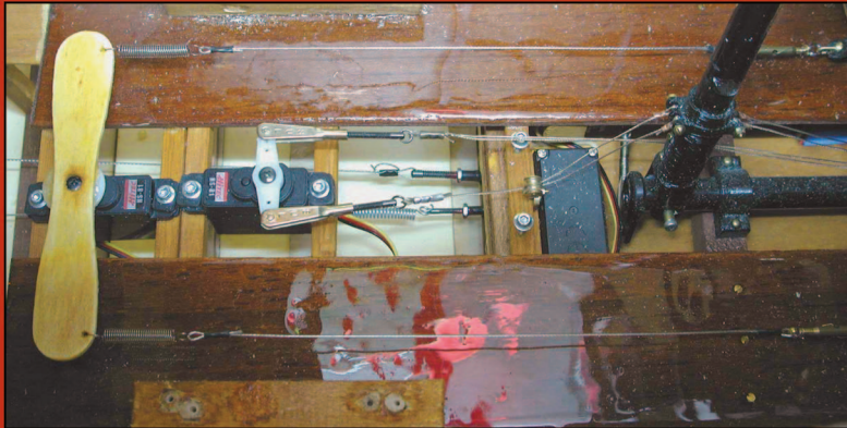
Movement mechanism and control system that activate the assembly movements are easily seen here. Note the springs used to protect the mechanisms components.
