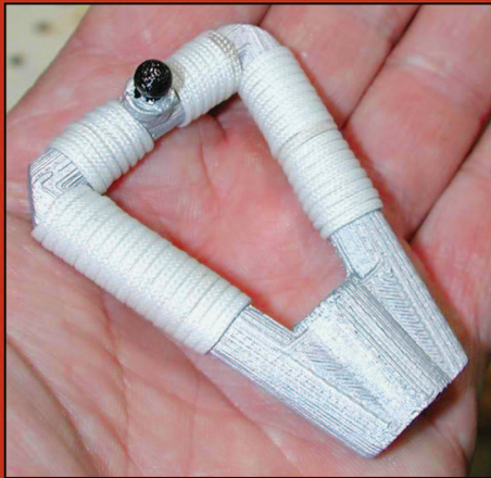
Control handle painted and the hand grip made from twine added. Note the ignition blip button.
