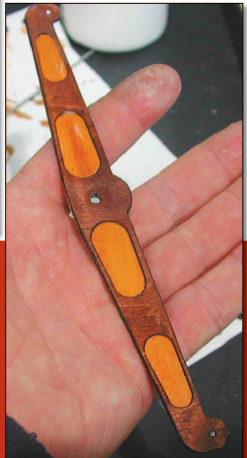
Completed rudder control bar with attachment points for control cables.
