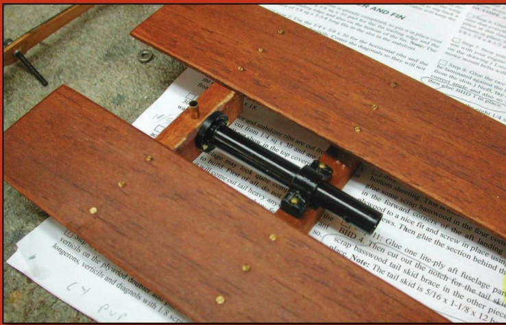
Cockpit floor and control assembly. Note the small brass wood screw.
