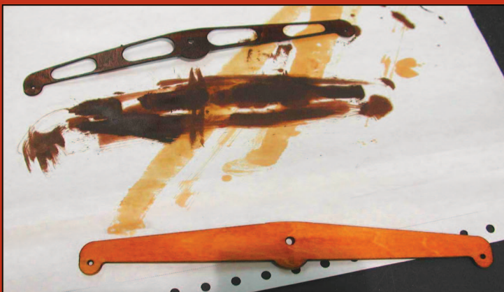
Two ply parts laminated to form the rudder control bar.
